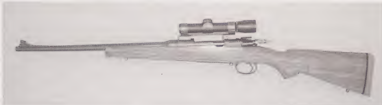
A .308 Mauser custom-built by master gunmaker Fred F. Wells. Note the quick-release Talbot scope mounts (which always allow a return to zero if the glass is removed) . . .
