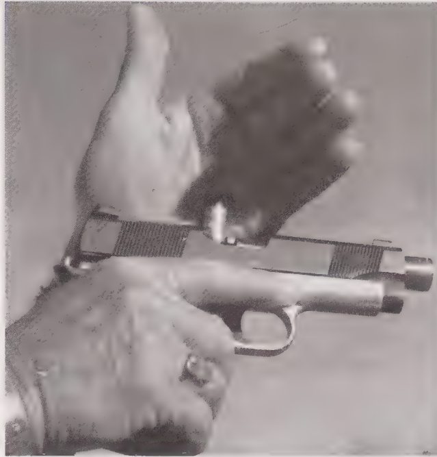
A "smokestack" malfunction in the process of being cleared by means of a rearward sweep with the support hand. Carry two guns!
