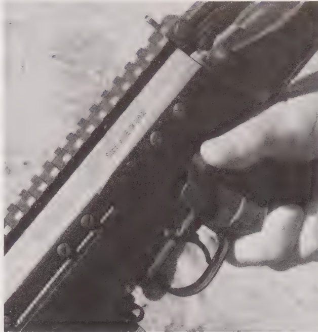
The thumb-operated safety about to be flipped "off" as an FN-FAL is mounted onto the target.
